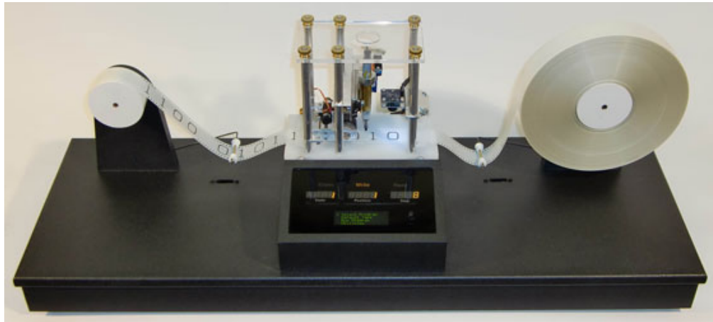
Figure 1: A physical Turing Machine built by Mike Davey supporting three symbols: 0, 1, and blank.
