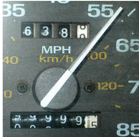
Figure 1: A mechanical car odometer [ mulears on Flickr ]
