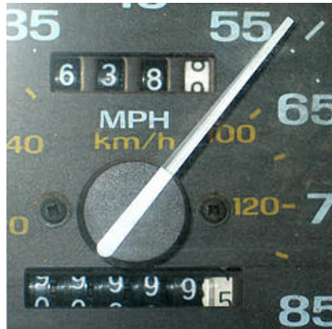
Figure 1: A mechanical car odometer [ mulears on Flickr ]
